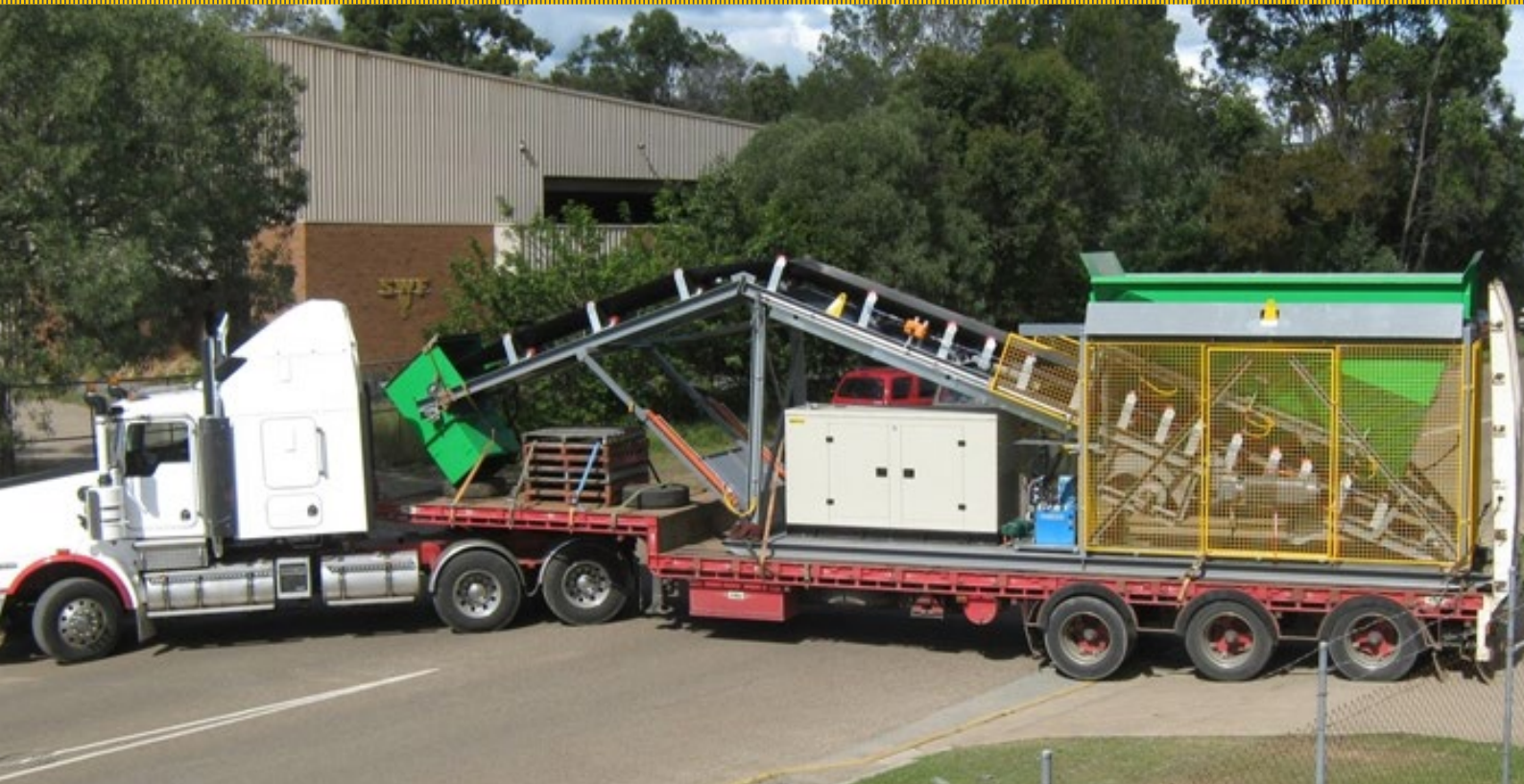
Road chip precoat plant being configured for transport
