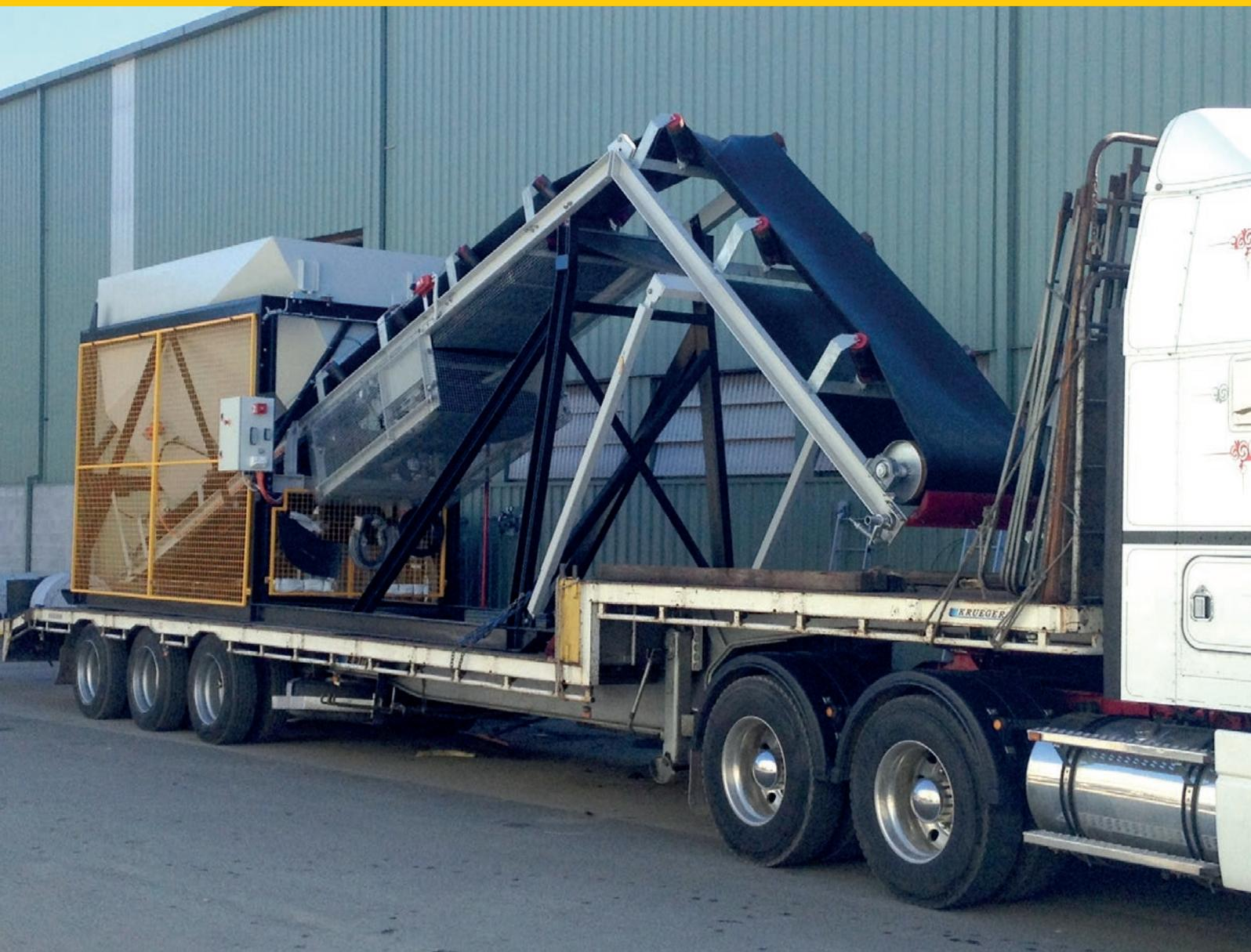
Auxiliary weigh hopper configured for transport
