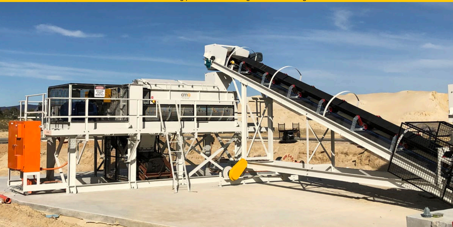
CMQ 600 tonnes per hour pugmill and radial conveyor
