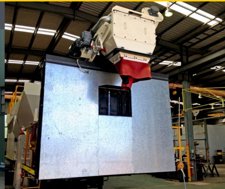
A folding truck loading bay cover – travelling position
