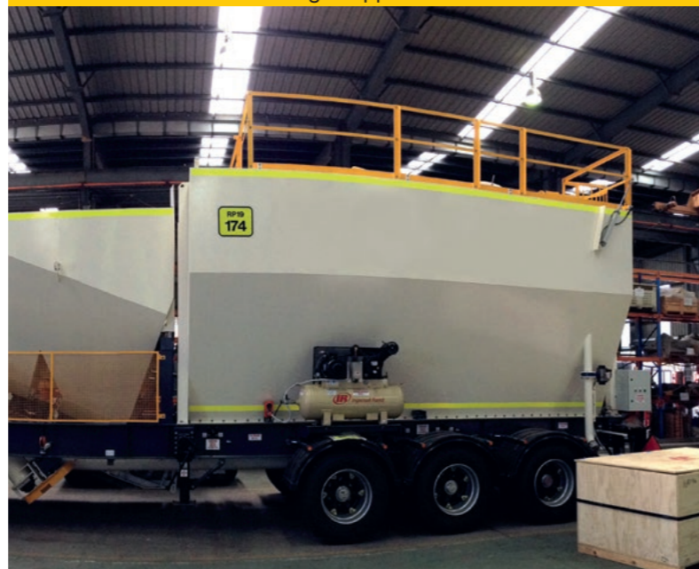
Pneumatically operated folding hand rails operated from the ground
