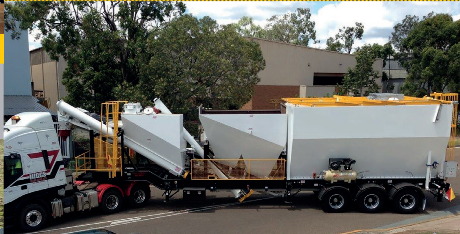
Portabatch being transported to site
