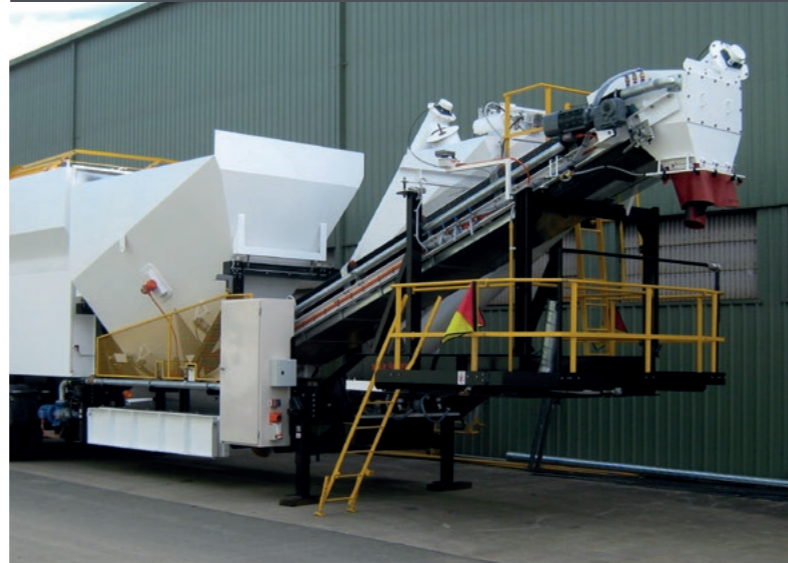
Platform and ladder for access to genset and CWH filter
