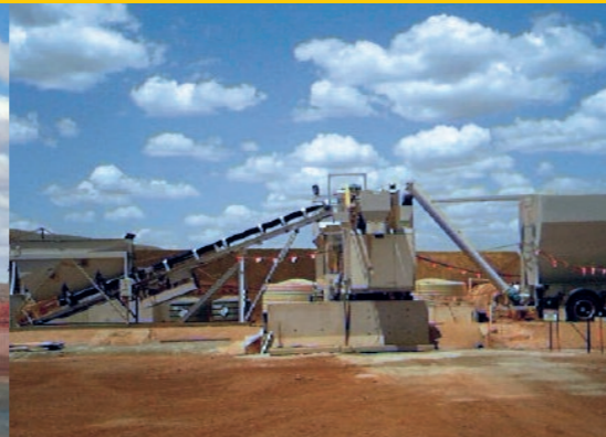
Newman Iron Ore Mine WA 1 Portabatch, 1 x 75T mobile silo 1 auxiliary weigh hopper
