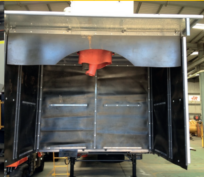
A folding truck loading bay cover – operating
