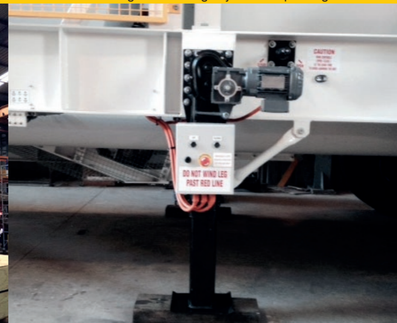
Electrically operated wind down leveling legs
