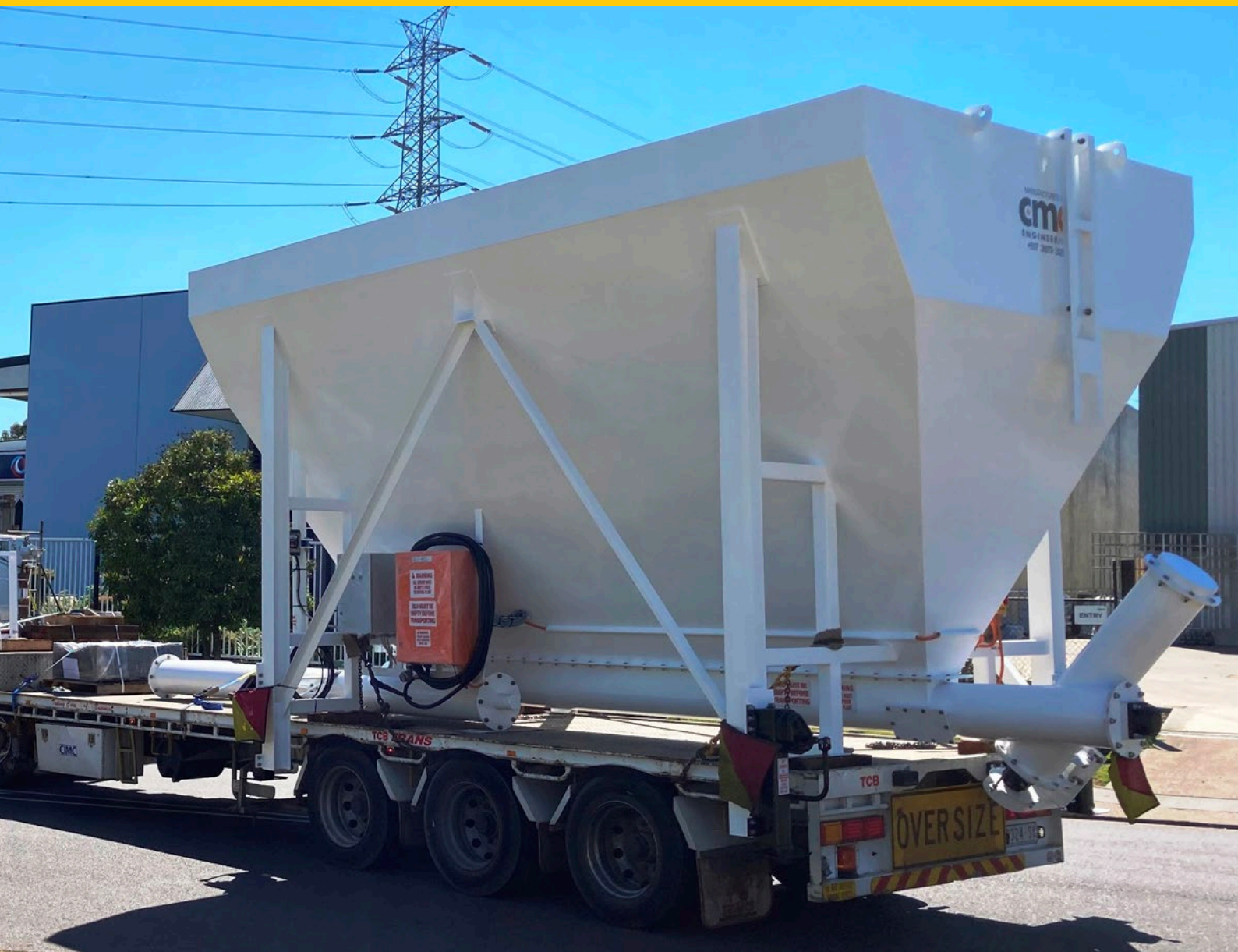
50T transportable cement silo
