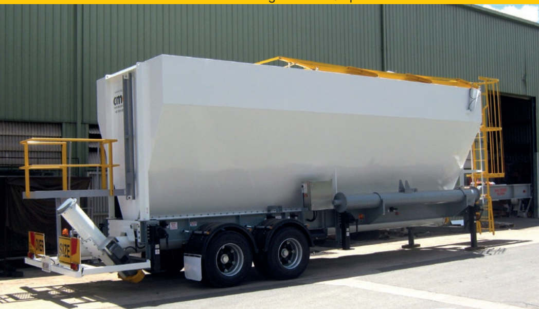
Cement silo configured for transport (rear side view)
