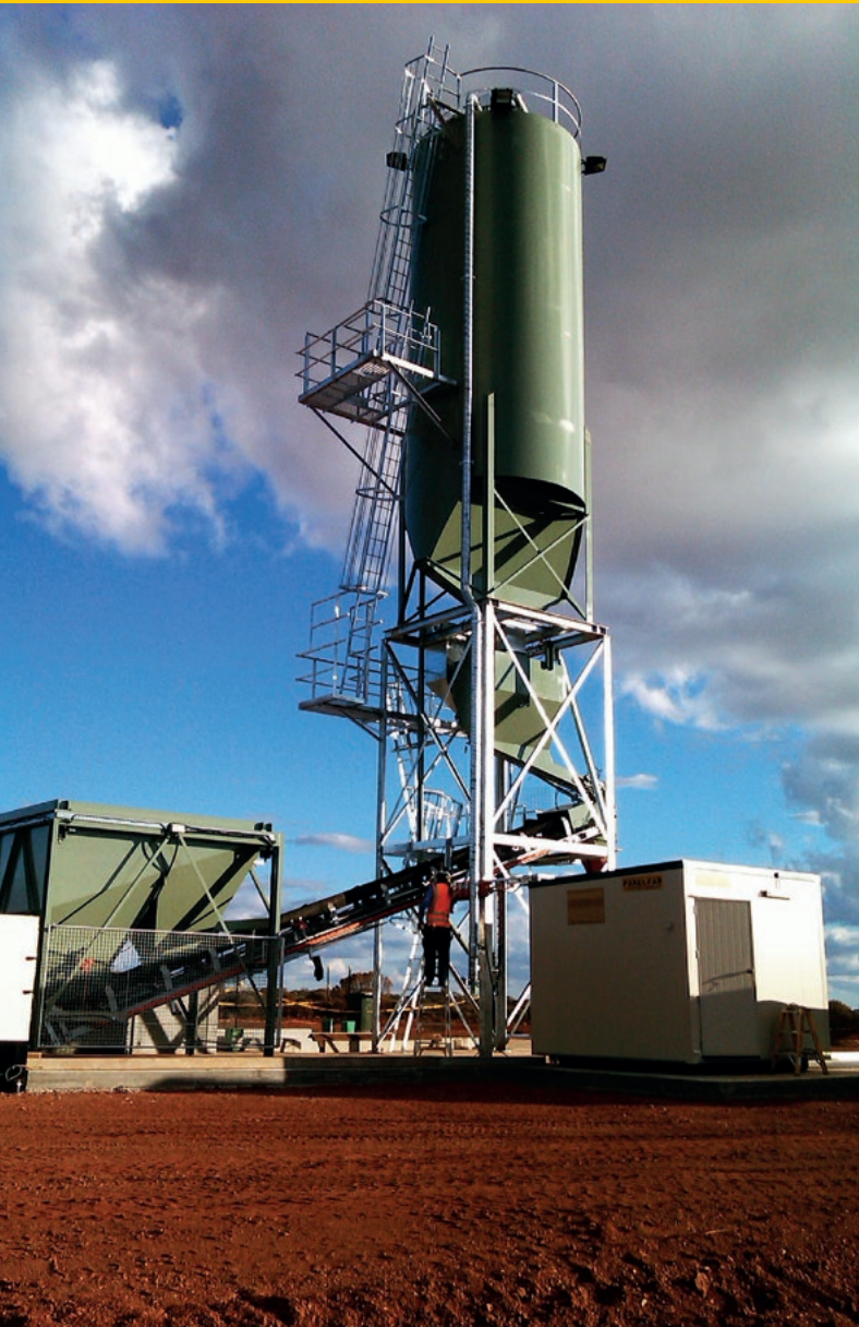
Front end loader fed plant 70m 3 /hr
