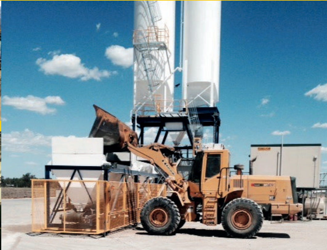
Low profile aggregate weigh hoppers – no ramp required
