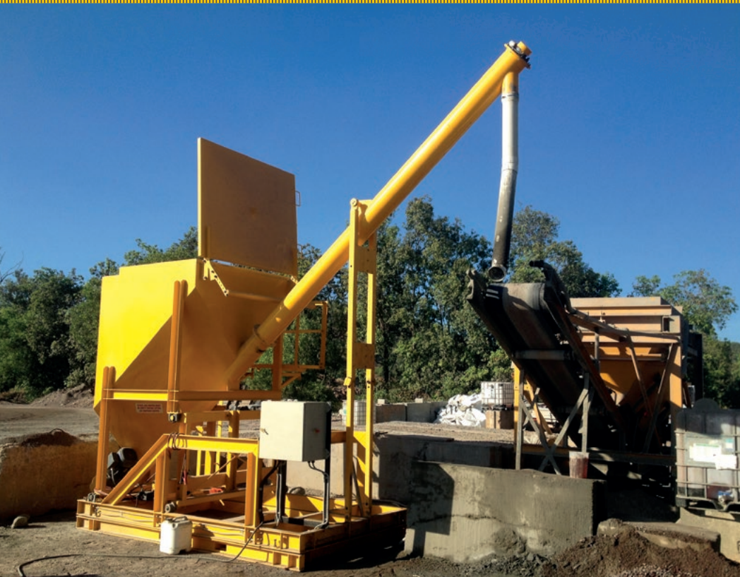
6T bag unloader feeding a throw in belt plant
