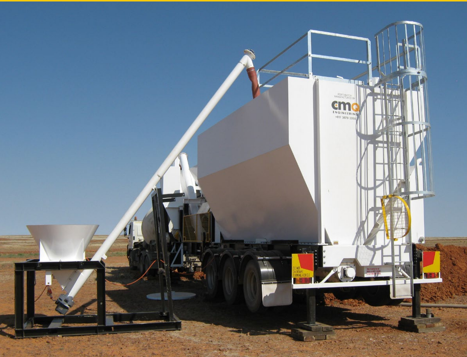
Bag unloader filling Portabatch silo
