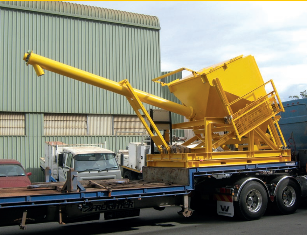
6T bag unloader folded for transport
