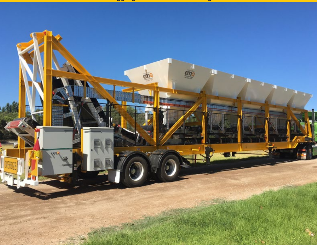
5-bin aggregate trailer being transported
