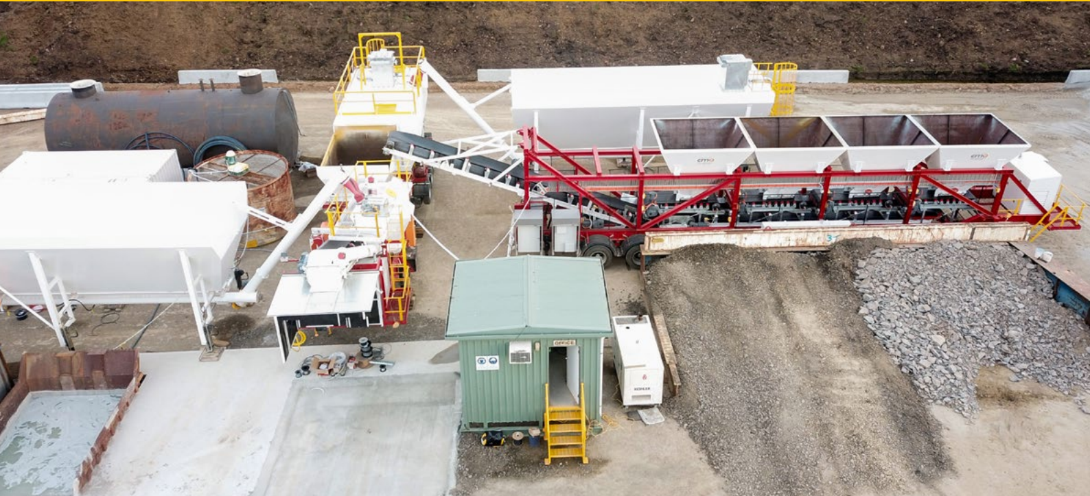
High production plant. Portabatch, 2 x 90T transportable silos, 4-bin aggregate feed trailer with belt weighers
