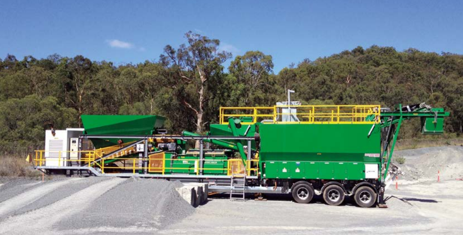
Mobile blending plant mobilised on site
