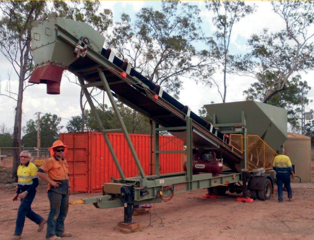
Transportable aggregate section in working position
