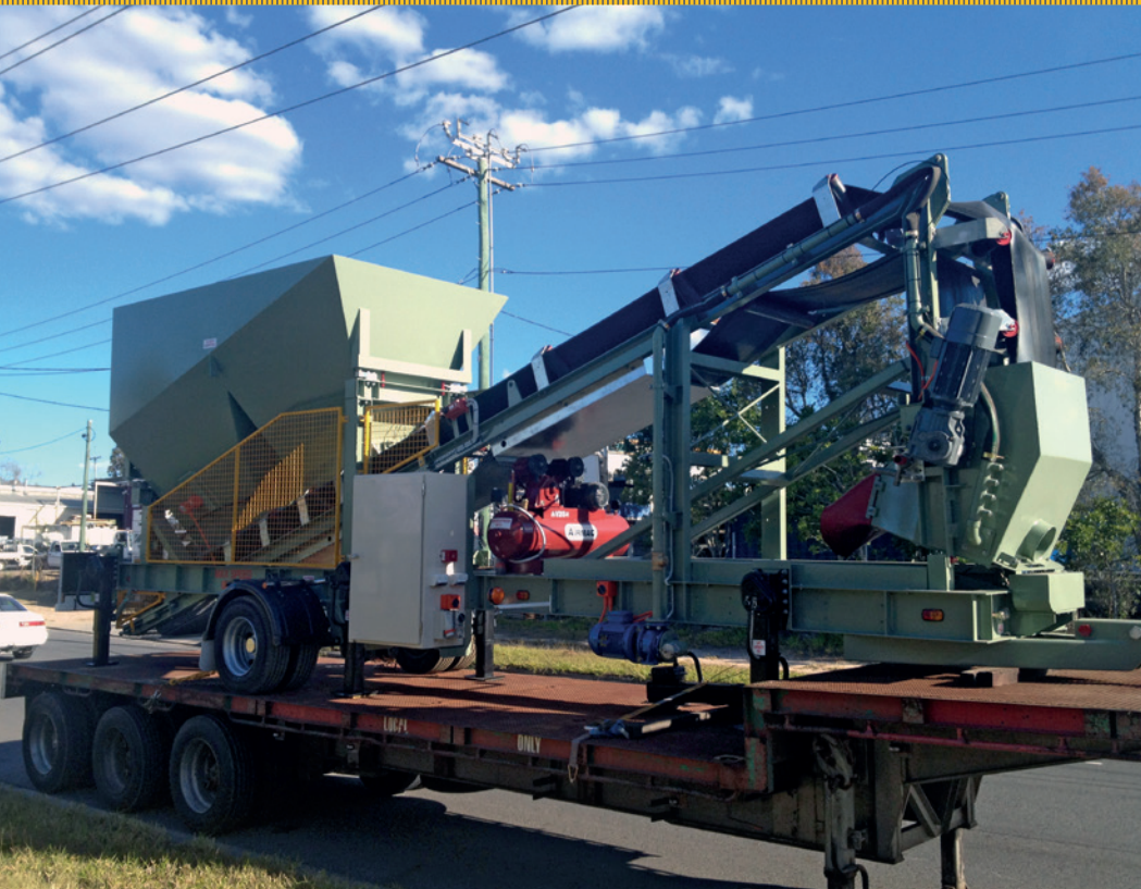
Transportable aggregate section in transport position ready for towing
