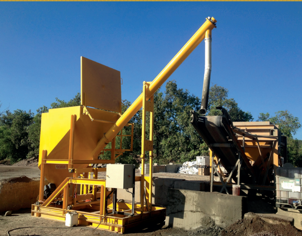
6T bag unloader feeding through into belt plant
