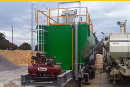
Silo and hopper in working position feeding mixture
