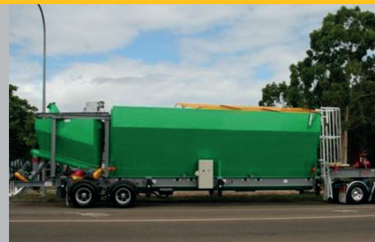
Side view configured for transport with lockable motor control centre
