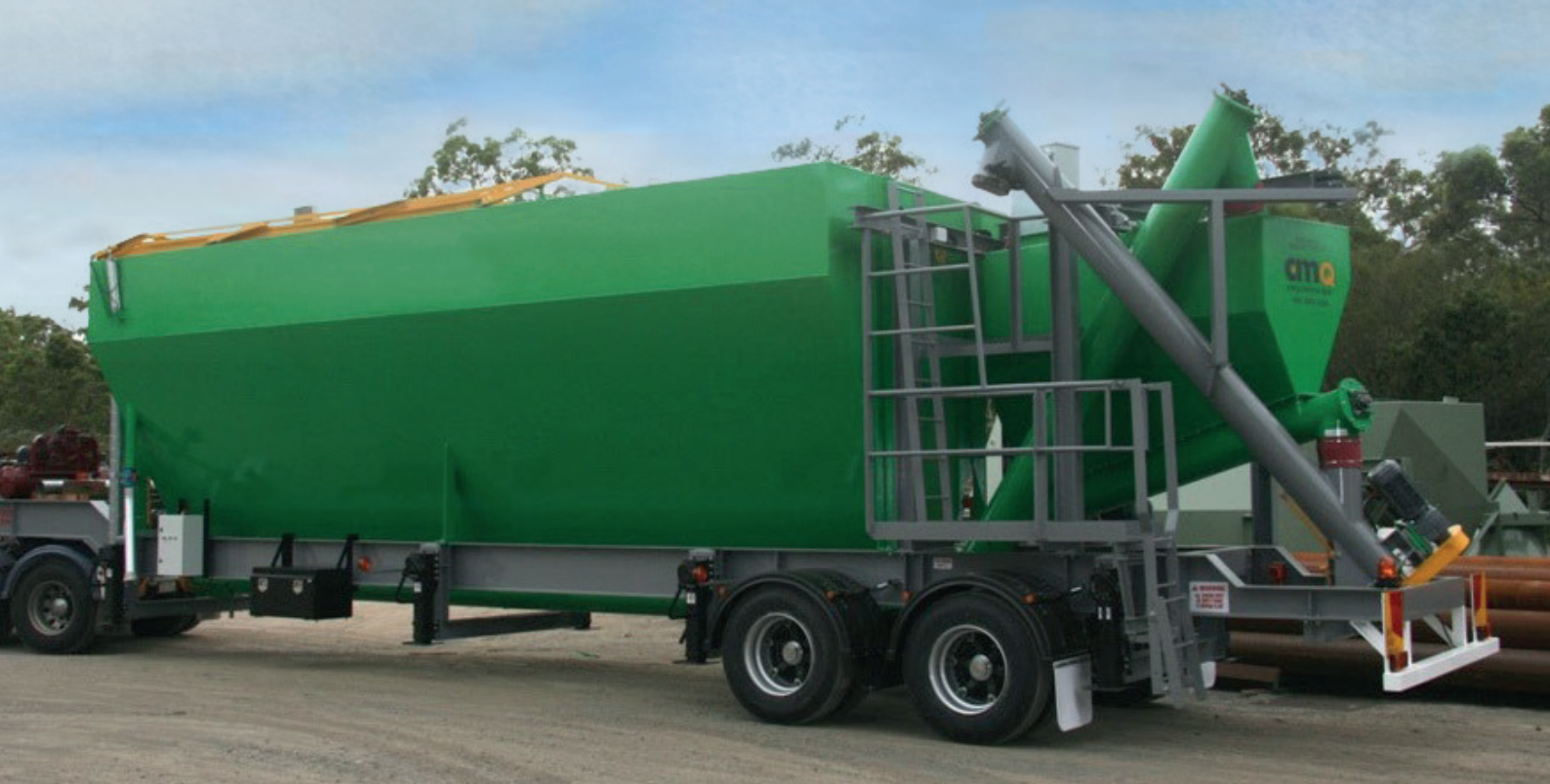
Mobile cement silo and hopper
